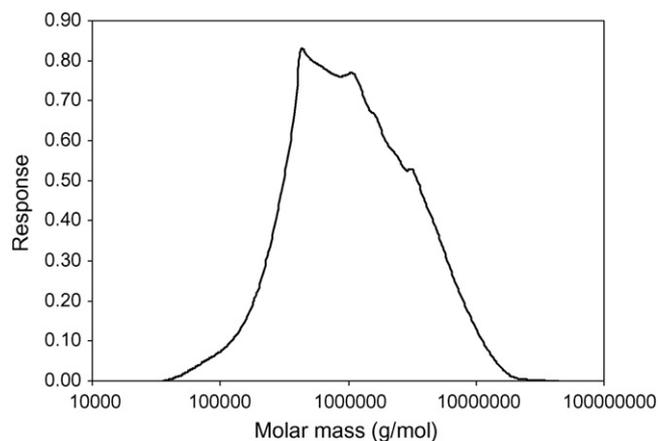
**Fig. 1.** Molar mass distribution of alginate used in this study, obtained from gel permeation chromatography: number average of molecular weight,  $M_n = 600$  kg/mol, weight average of molecular weight,  $M_w = 1900$  kg/mol, polydispersity index  $\text{PDI} = M_w/M_n = 3.2$ .
