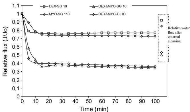
Fig. 9. Normalized flux during ultrafiltration of dextran–myoglobin mixture solution (single-solute solutions for comparison) using PES-based UF membranes at a trans-membrane pressure of 100 kPa (dextran concentration 1 g/L, MYO concentration 0.1 g/L, pH ~7). Water fluxes after external cleaning with water, relative to initial water flux are also included.
