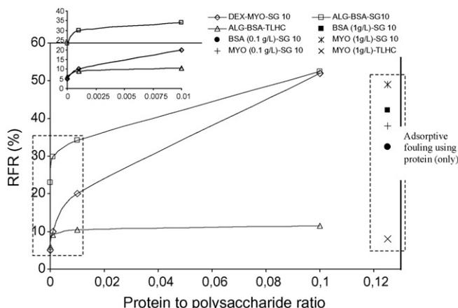
Fig. 5. Influence of protein/polysaccharide ratio on relative flux reduction for unmodified and TLHC membranes with a cut-off of 10 kg/mol. Polysaccharide concentration was fixed at 10 g/L and adsorption time was 3 h. RFR data for after static adsorption using protein (only) solution (either 1 or 0.1 g/L) are included for comparison.
