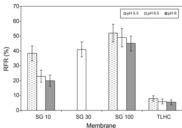
**Fig. 2.** Effects of membrane characteristics and pH value of solution on relative flux reduction during adsorptive fouling (alginate concentration 10 g/L, adsorption time 3 h). For study of pH effect, the alginate was dissolved in phosphate buffer (0.05 M); thereby the total ionic content could be kept almost constant. The error bars represent standard deviation.
