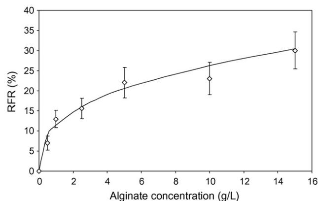
**Fig. 3.** Influence of alginate concentration on relative flux reduction after static adsorption (membrane SG 10, pH 6.5, adsorption time 3 h). The error bars represent standard deviation.
