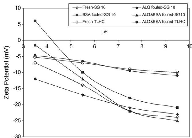
**Fig. 6.** Zeta potentials as a function of pH (at 0.001 mol/L KCl) for membrane SG 10 and TLHC membranes, before and after exposing for 3 h to protein (1 g/L), polysaccharide (10 g/L), or polysaccharide-protein (10/1 g/L) mixture solution.
