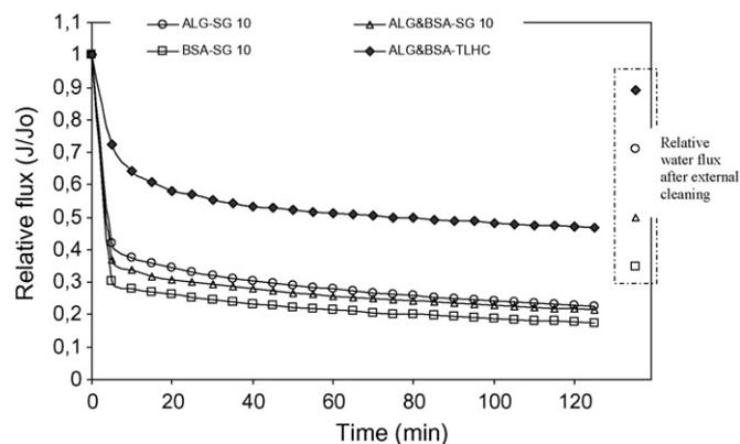
**Fig. 8.** Normalized flux during ultrafiltration of alginate-BSA mixture solution (single-solute solutions for comparison) using PES-based UF membranes at a trans-membrane pressure of 100 kPa (alginate concentration 1 g/L, BSA concentration 0.1 g/L, pH  $\sim 7$ ). Water fluxes after external cleaning with water, relative to initial water flux are also included.
