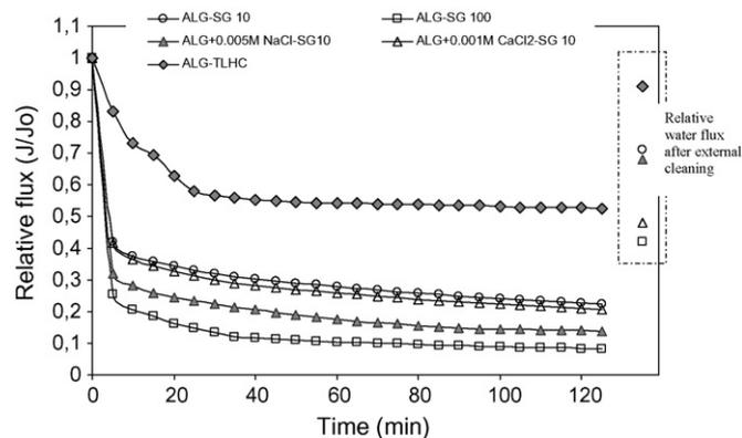
**Fig. 7.** Normalized flux during ultrafiltration of alginate solutions using PES-based UF membranes at a trans-membrane pressure of 100 kPa (initial alginate concentration 1 g/L in water, NaCl and CaCl<sub>2</sub> were added in two experiments as indicated). Water fluxes after external cleaning with water, relative to initial water flux are also included.
