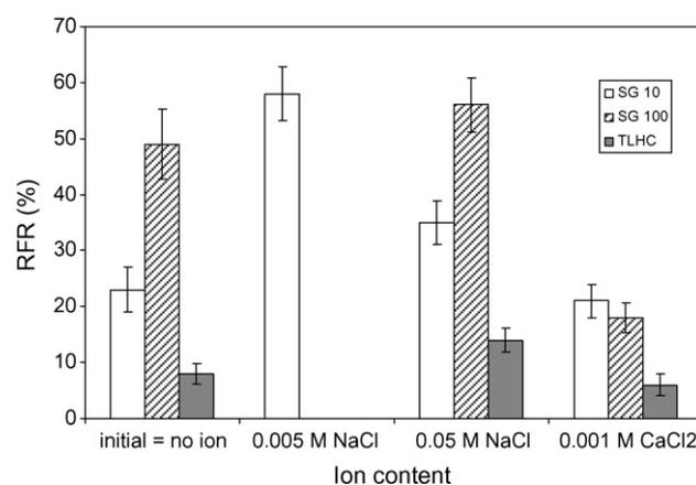
**Fig. 4.** Relative flux reduction of three different membranes after static adsorption (3 h) by using alginate (10 g/L) in aqueous solutions with different ionic environments. The error bars represent standard deviation.
